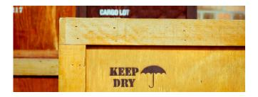
Crating is more secure than palletizing an engine, and will reduce the likelihood of damage, but crates can be more difficult to handle and may be more expensive to produce.
